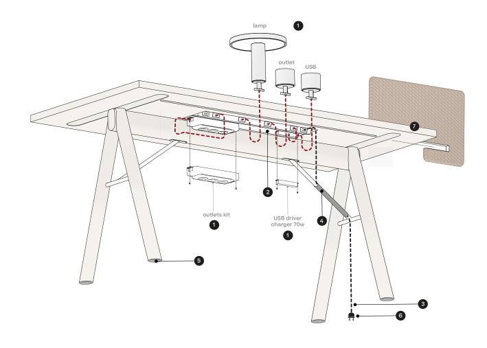
1 Electrical accesories 2 Connectivity system integrated 3 Power cable 4 Cable holder clip 5 Adjustable table levelers 6 Worldwide electrical plugs 7 Screen divide
