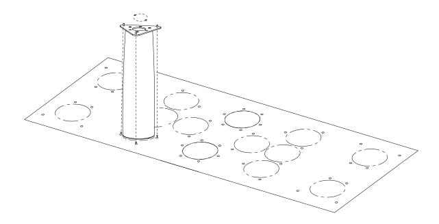
Unscrew the center leg plates and screw on the dual mounting kit.
