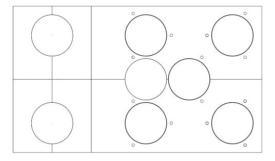
Once all the legs are placed, rotate them until they align with the small holes in the templates.
