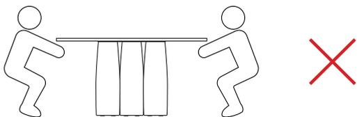
The packed top must always be handled and transported vertically, the tops must never be transported horizontally.
