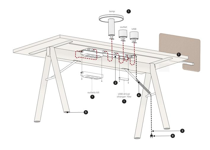
1 Electrical accesories 2 Connectivity system integrated 3 Power cable 4 Cable holder clip 5 Adjustable table levelers 6 Worldwide electrical plugs 7 Screen divid
