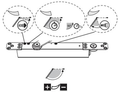
**i** Tighten or untighten the screws to their corresponding tightening torque between 1 to 2 Nm by hand.
