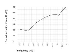
R<sub>w</sub> (C;Ctr)=46(-2;9)dB R<sub>A</sub> =44dBA
