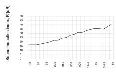
R<sub>W</sub> (C;Ctr)=32(-0;4)dB R<sub>A</sub> =32dBA
