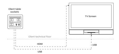
This wiring, shown in the image above, must be installed from the TV+SoundBar panel, through the client's raised floor, to where the equipment for controlling the peripheral devices must be located. Our pavilion does not have a raised access floor for routing cables.
