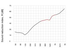
R<sub>W</sub> (C;Ctr)=38(-2;-8)dB R<sub>A</sub> =36dBA
