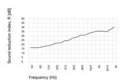
R<sub>W</sub> (C;Ctr)=32(-0;4)dB R<sub>A</sub> =32dBA
